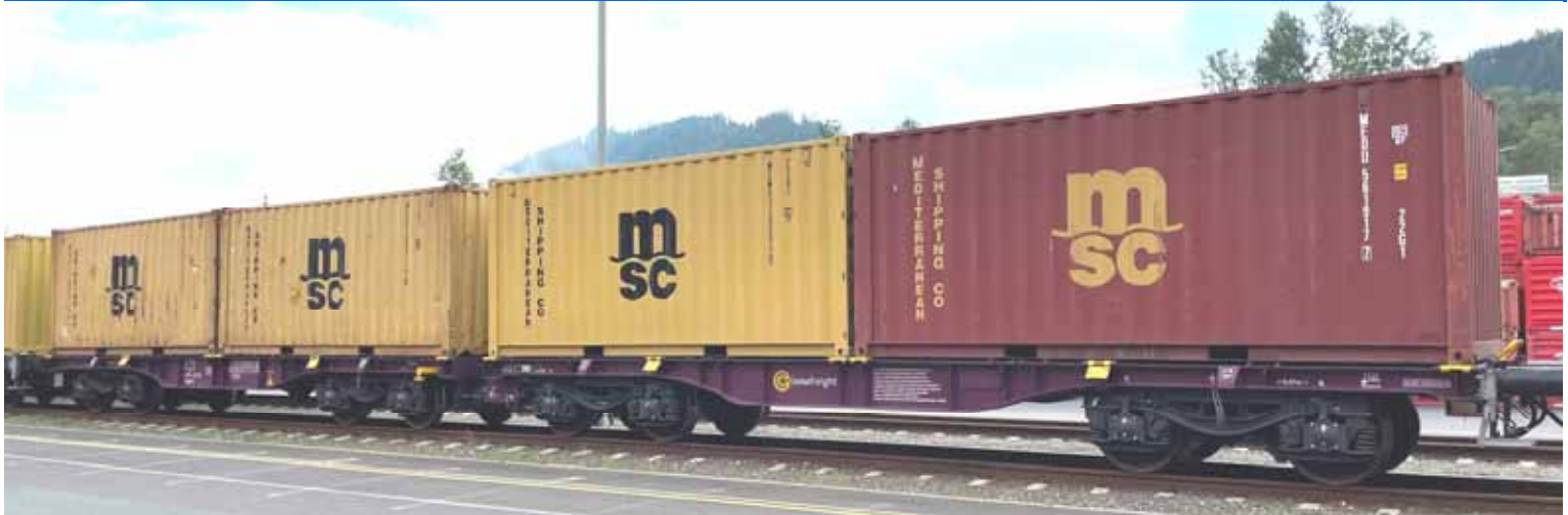
Ref n° : 90.503 Purple innofreight car loaded with 4 yellow 20ft containers MSC (3 Yellow + 1 Brown)
